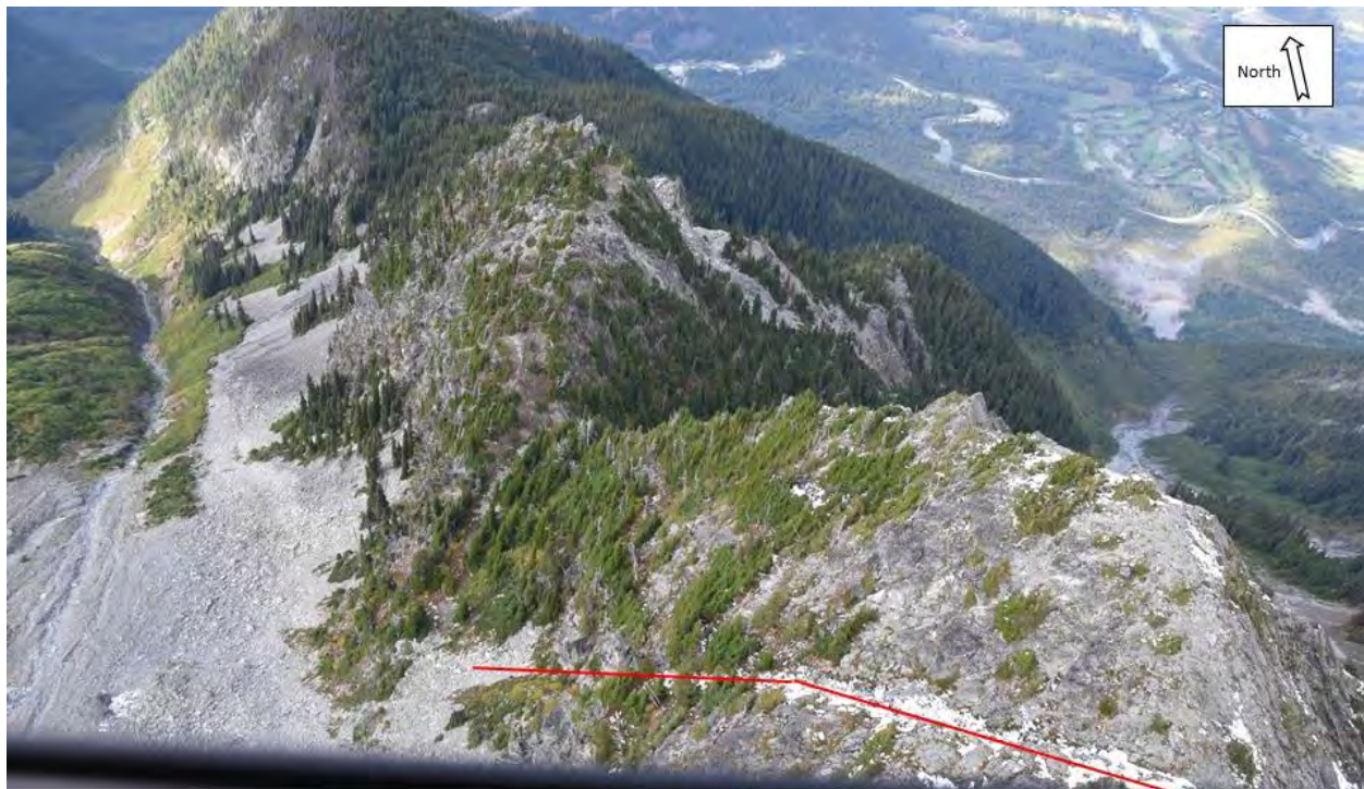
Photograph 40 Lineament (red line) marking the upper extent of potential Source ID 14.
