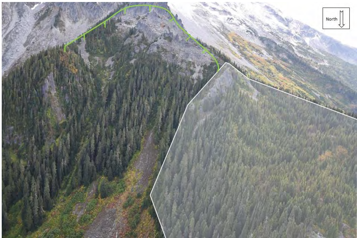
Photograph 19 Upper part of Source ID 4, where tension cracks are developing in the forested area (white transparent polygon) and scar of a past landslide event (green line) where more unstable ground forms Source ID 16 (see Photograph 21).
