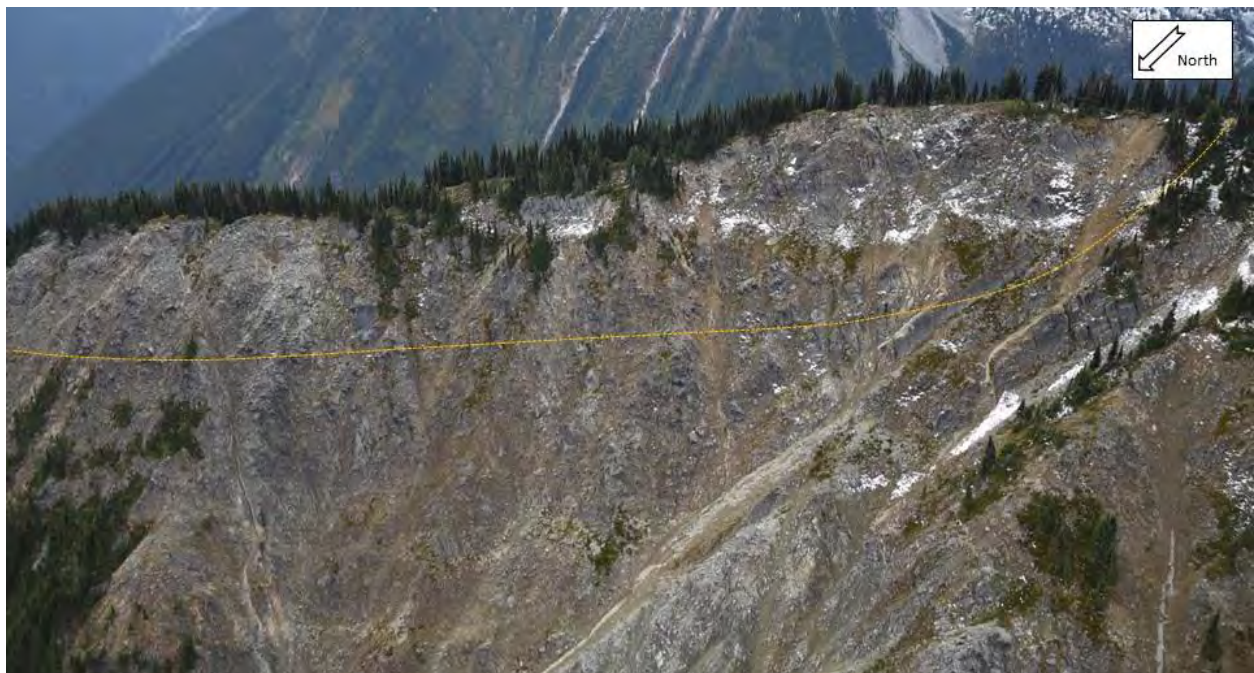
Photograph 14 Source ID 2a and the inferred location of its basal sliding surface (orange dashed line).
