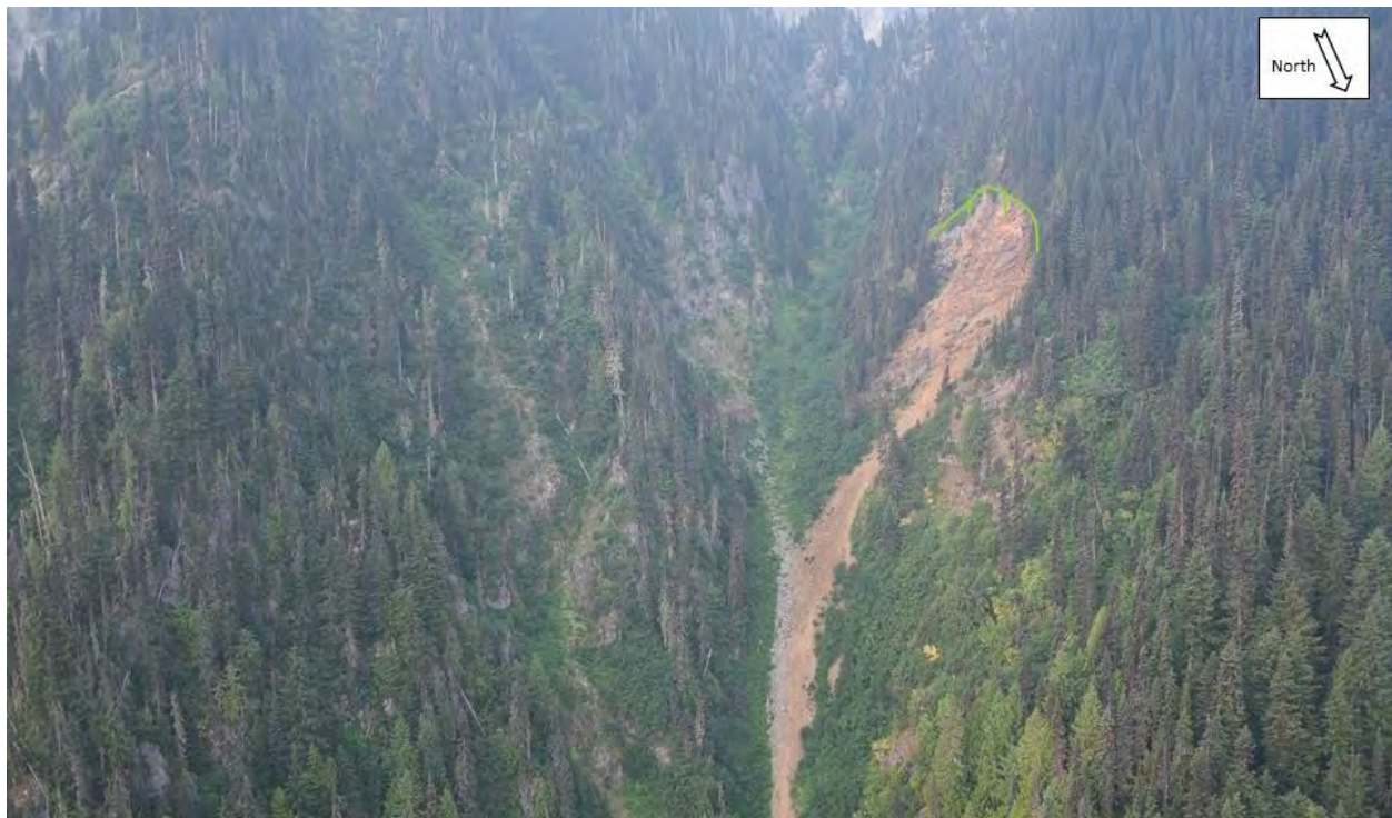
Photograph 27 Rock and debris slide in the easternmost watershed. The green line shows the scar.
