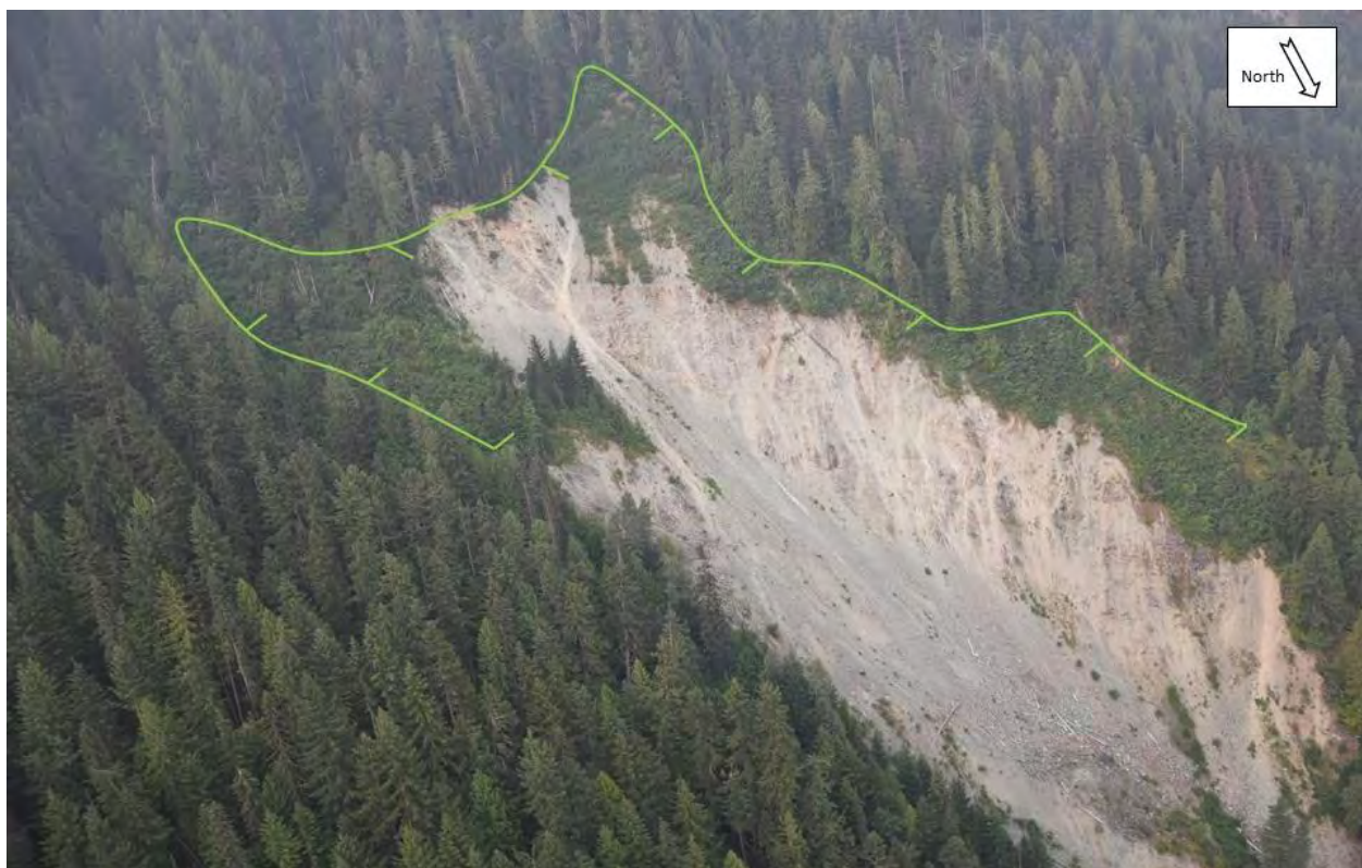
Photograph 42 Rock and debris slide showing re-vegetation of the scar of the event which occurred between 1948 and 1969. Possible retrogression of this landslide represents Source ID 5.
