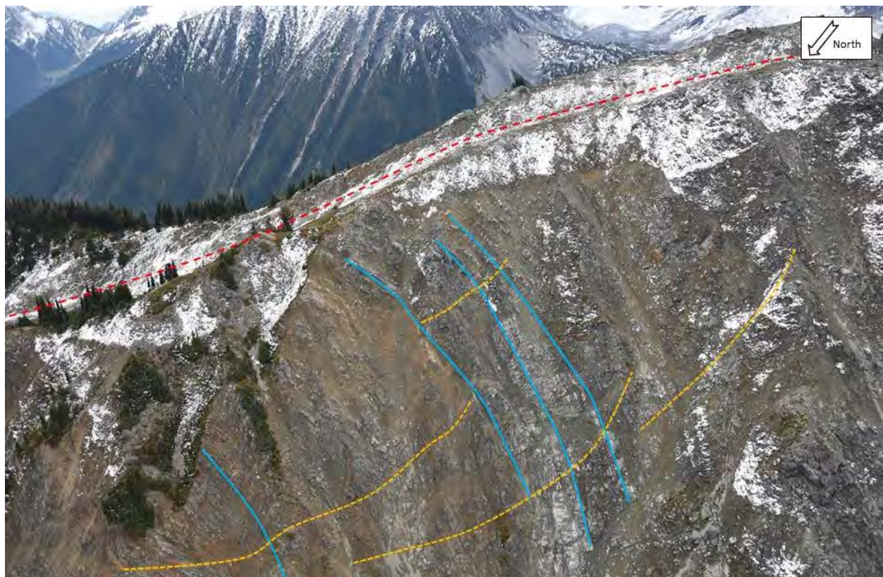
Photograph 9 Section of Source ID 1b showing the upper extent along a counter-slope scarp (red dashed line), interpreted basal sliding surfaces (orange dashed lines), and inflexed foliation planes (blue lines).
