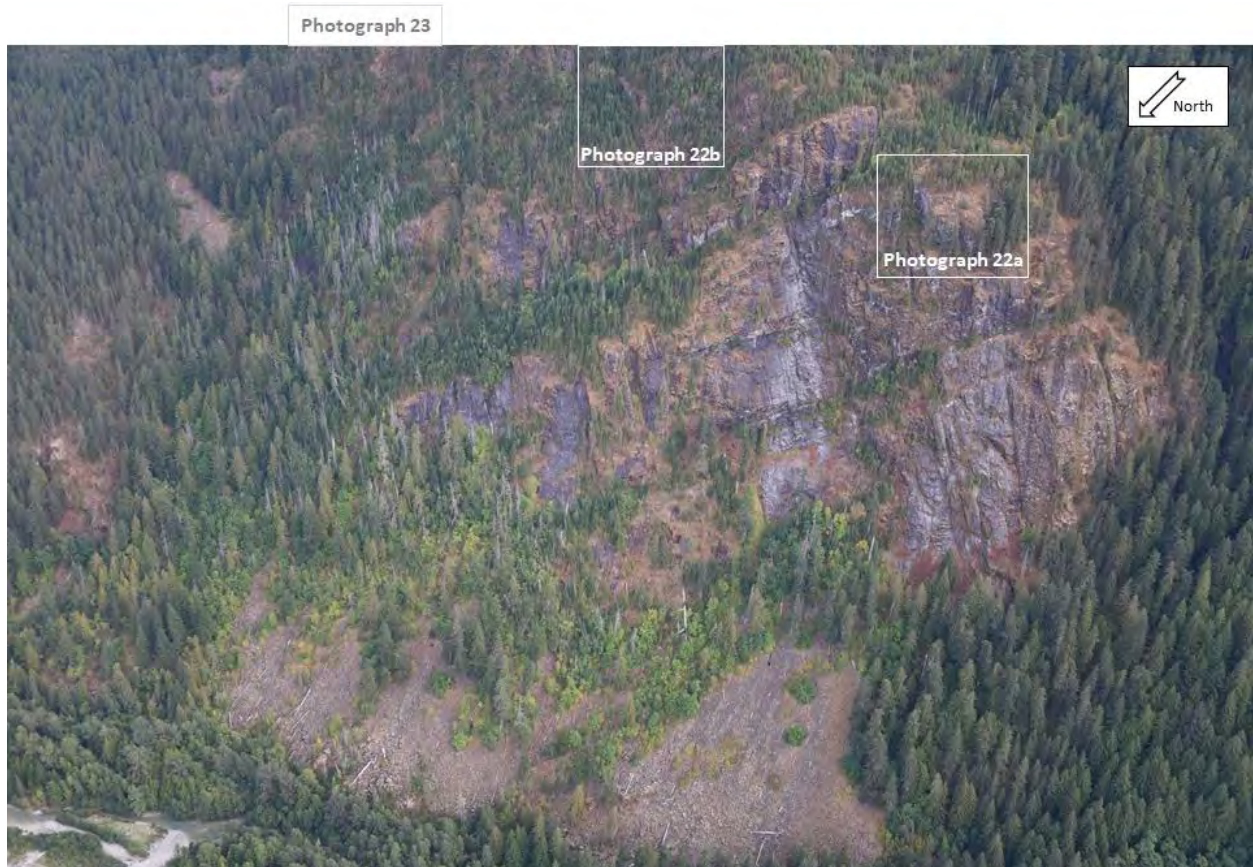
Photograph 24 DSGSD (Source ID 13) showing rock fall debris (weathered and covered with vegetation) at the base of a rock slope. Green River flows at the toe of the debris.
