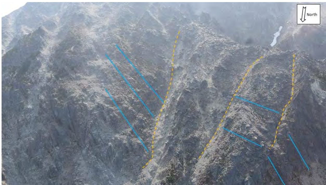
Photograph 36 Disturbed mass along the crest separating Watershed C and D. The orange dashed line shows interpreted basal sliding surfaces constrained by the location where undisturbed foliation planes are tilted (blue lines).
