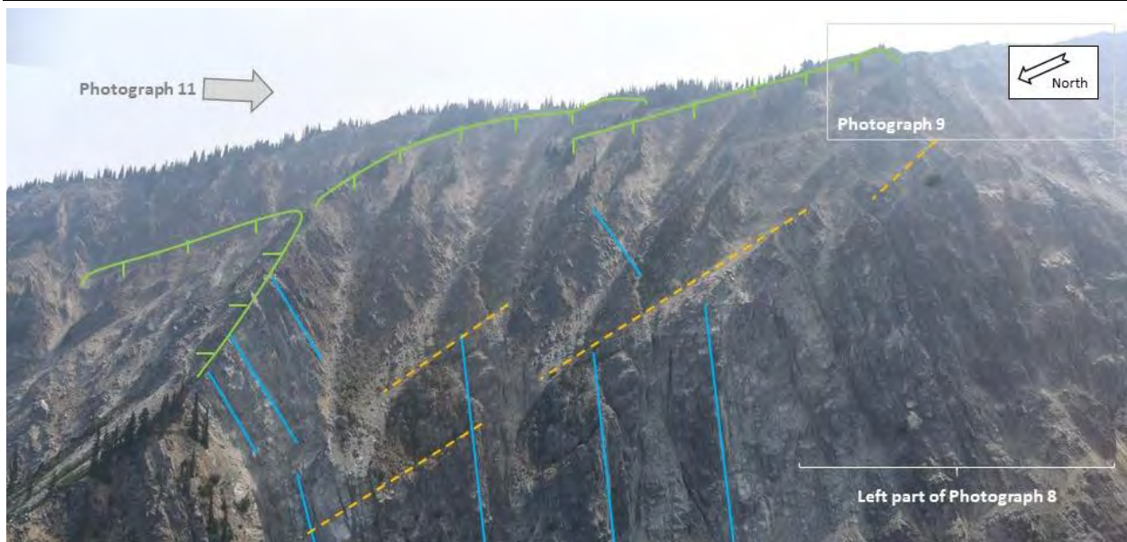
Photograph 10 Disturbed mass (Source ID 1b) with interpreted basal sliding surfaces (orange dashed line) constrained by the location where undisturbed foliation planes become tilted (blue lines). Green lines show scars of small landslides initiating on the edge of the mass.
