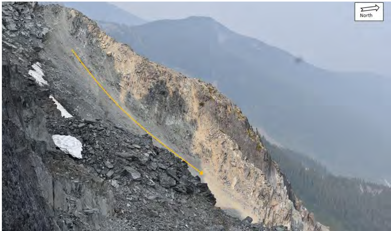
Photograph 29 Scar of the small disturbed mass, whose failure is assumed to have been triggered by a rock fall event, as explained in Photograph 28.
