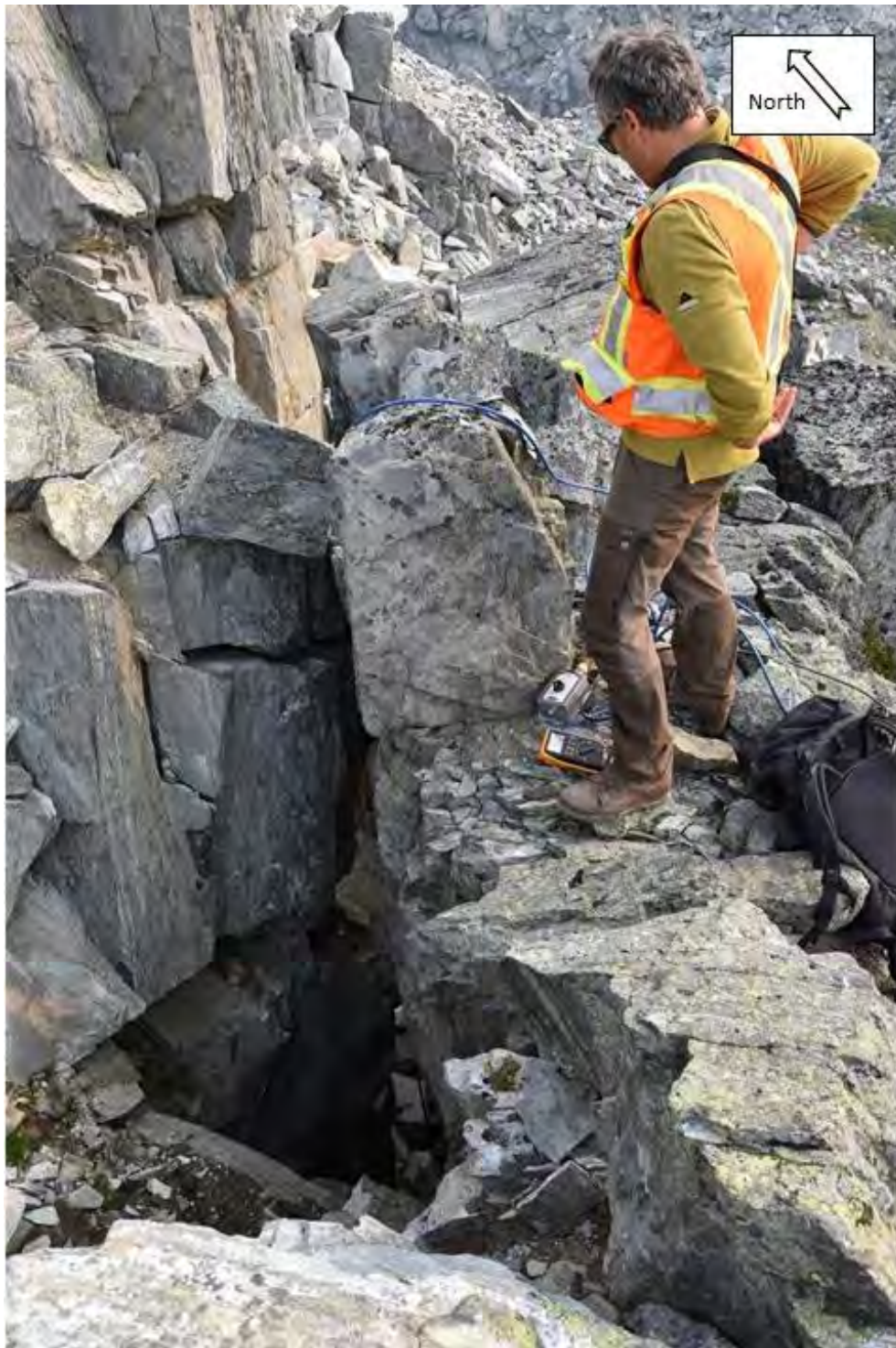
Photograph 51 Crack at Station 17-01 where the thermistor was used to generate a temperature profile.
