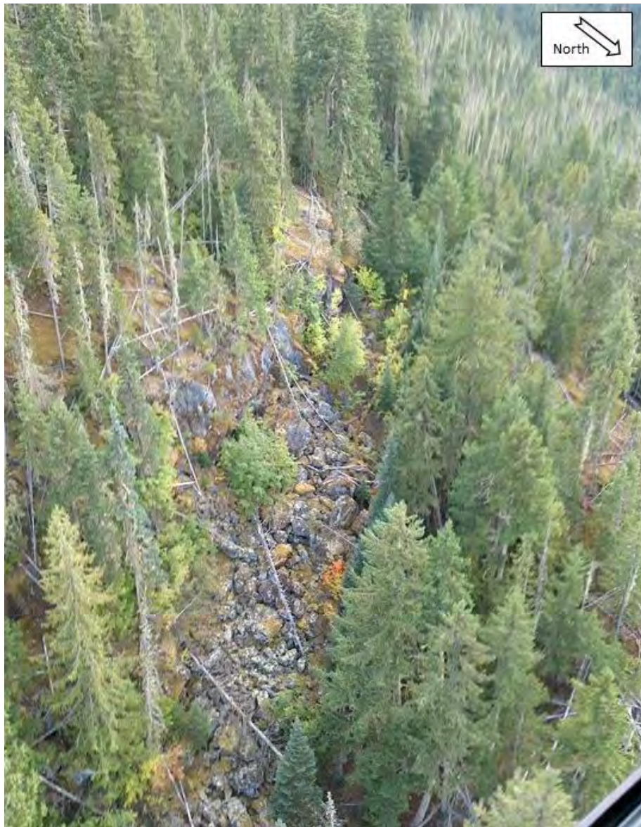
Photograph 23 Wide northeast trending tension crack filled with rock blocks and vegetation, and marking the upper limit of potential Source ID 13. The surface of the blocks is weathered and appears to be covered with lichen.
