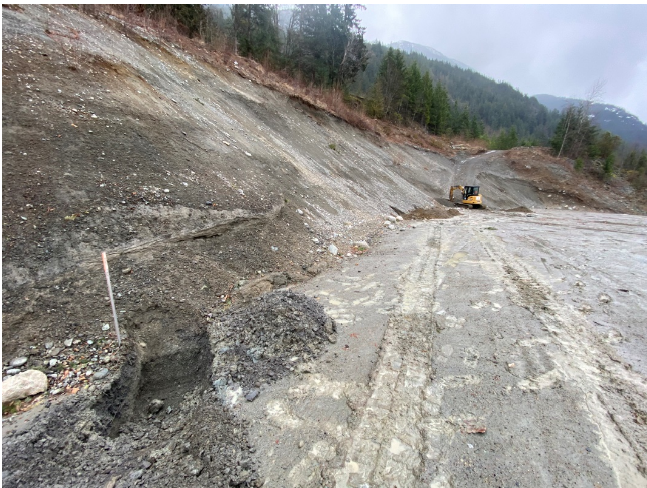
Figure 3 - Testpit 4 Looking South (Area 2). Native sand and gravel is visible along the slope
