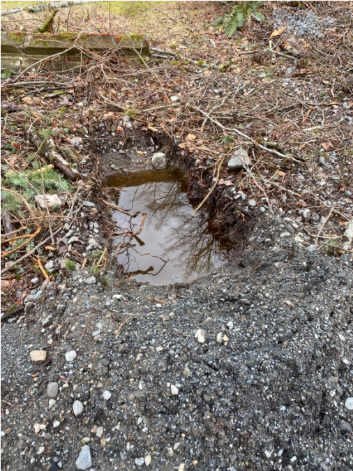
Figure 1 - Photo showing Test pit 1 – Note perched water table
