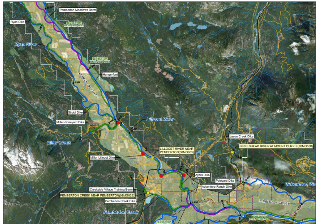
Figure 24 – Flood Zones and Dike Infrastructure in the Lillooet River Lower Reach (Source: NHC 2018)
