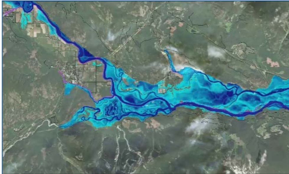
Figure 5 – Projected inundation from a 200-Year Flood event on the Lillooet River Lower Reach, depicting the Village of Pemberton, Pemberton Meadows, Mount Currie and the Pemberton Fringe in Electoral Area C (Source: NHC, 2019)
