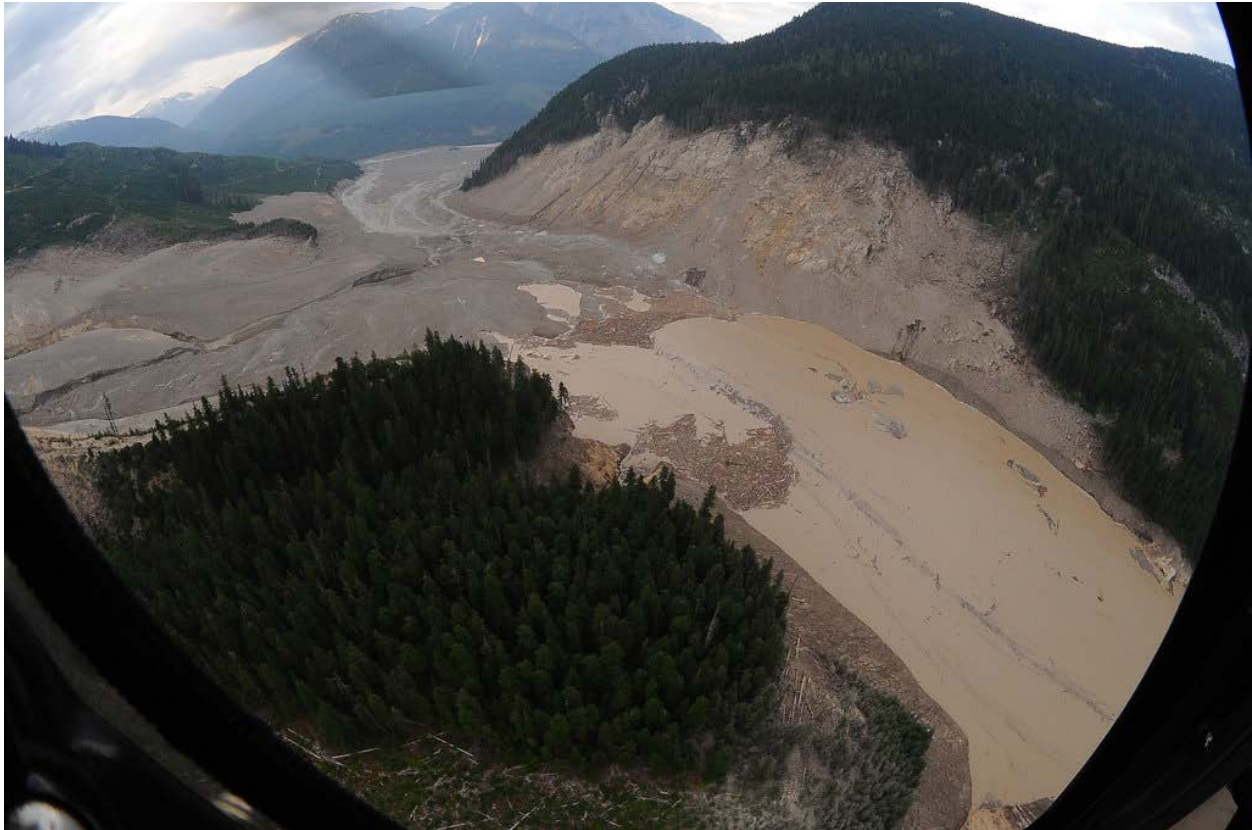
Figure E-16. Landslide dam on Meager Creek from the August 6, 2010 rockslide-debris flow from Capricorn Creek. The dam impounded Meager Creek for some time. Photo by D. Steers.
