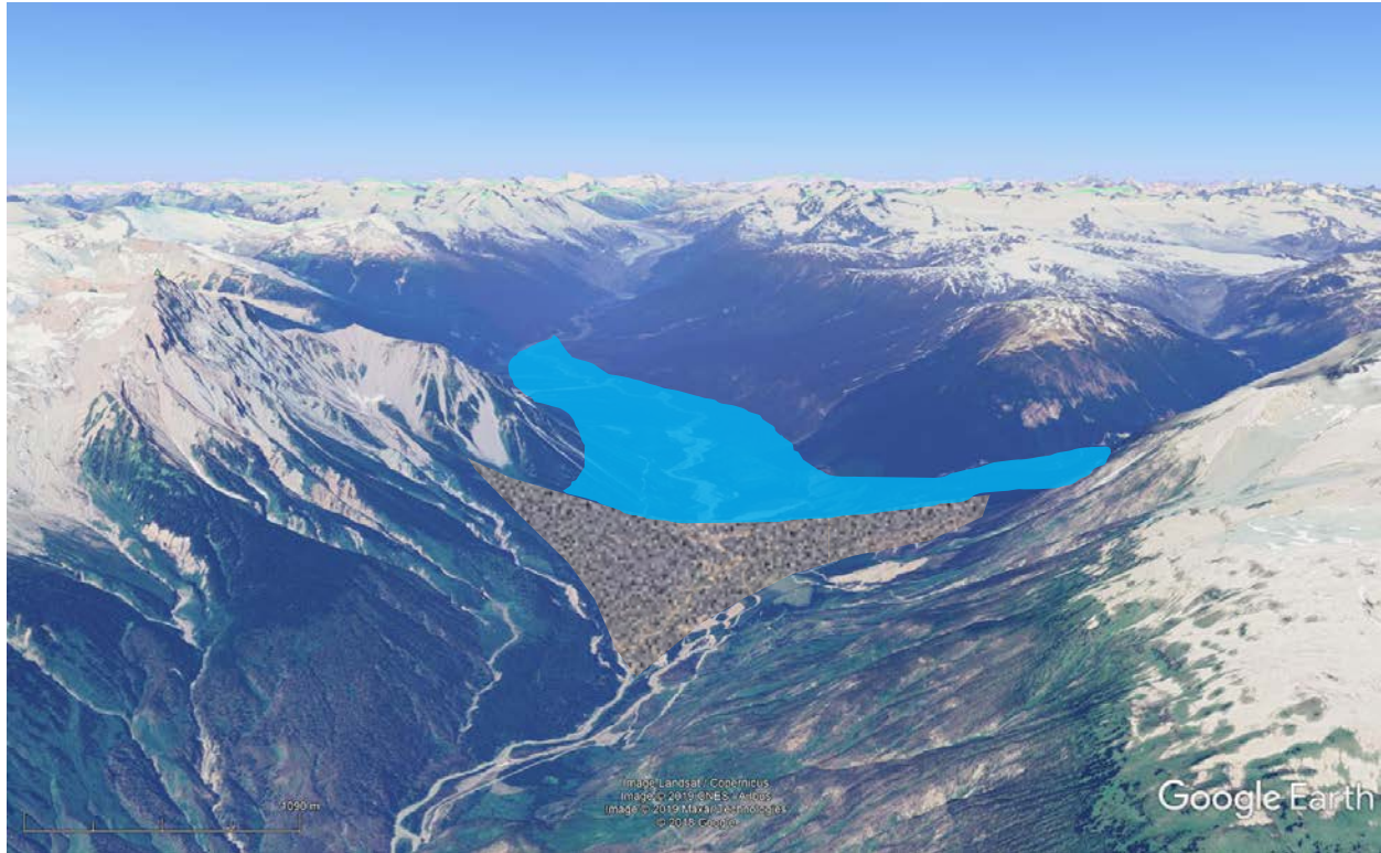
Figure F-1. Upper Lillooet River Valley with Plinth Peak on the left. The sketched outline shows a past landslide dam and the possible extent of a rock avalanche from the north flanks of Plinth Peak.
