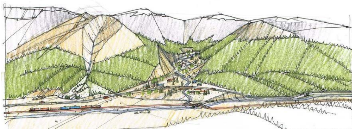
Figure E-3. Typical steep and low-gradient fans feeding into a broader floodplain. On the left a small watershed prone to debris flows has created a steep fan that may also be subject to rock fall processes. On the right a larger watershed prone to debris floods has created a lower gradient fan. Development and infrastructure are shown to illustrate their interaction with steep creek geohazard events. Artwork: Derrill Shuttleworth.
