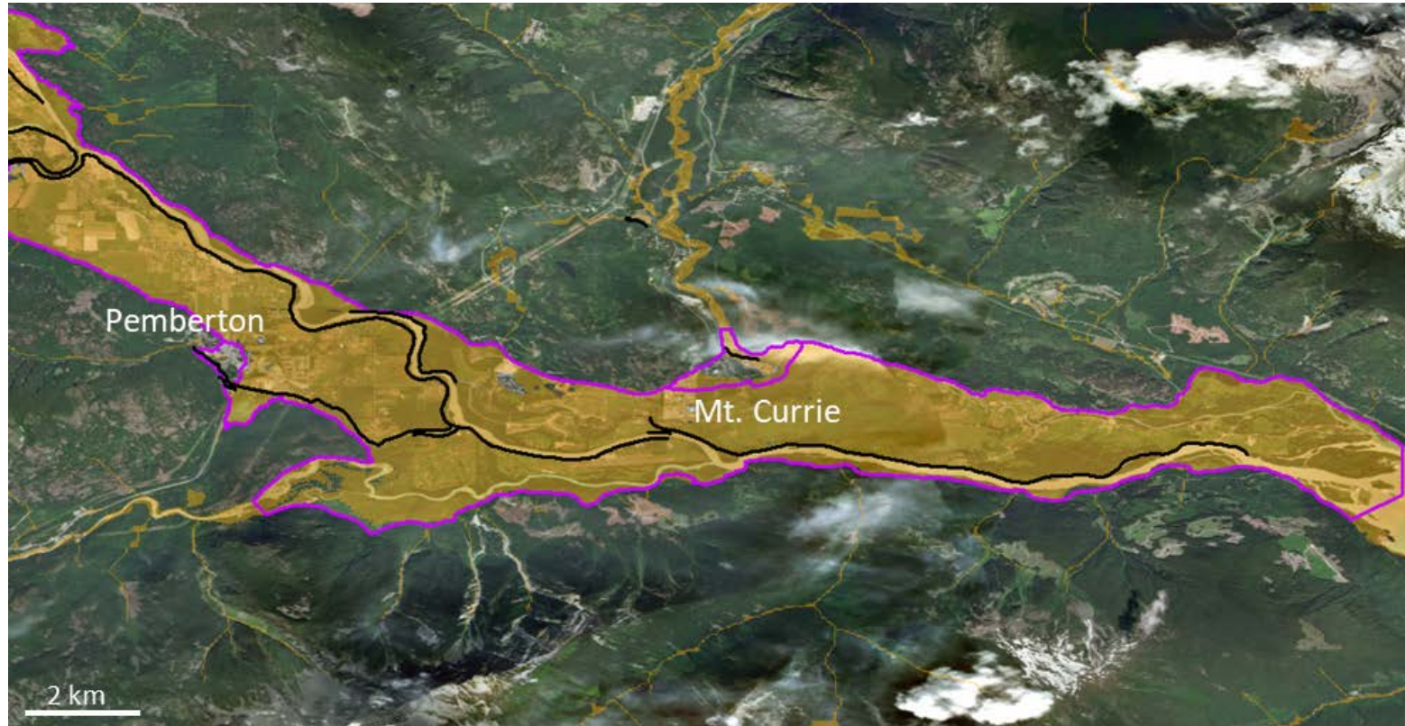
Figure D-3. Example spatial sources used to identify clear-water flood hazards in the SLRD including historical floodplain mapping (purple outlines) and predicted floodplain extents for streams and lakes without existing floodplain mapping (transparent orange areas). Locations of known flood protection structures (black line) were inventoried but not prioritized. Refer to Section D.2.4 for a description of the methods used for predicting floodplain extents.
