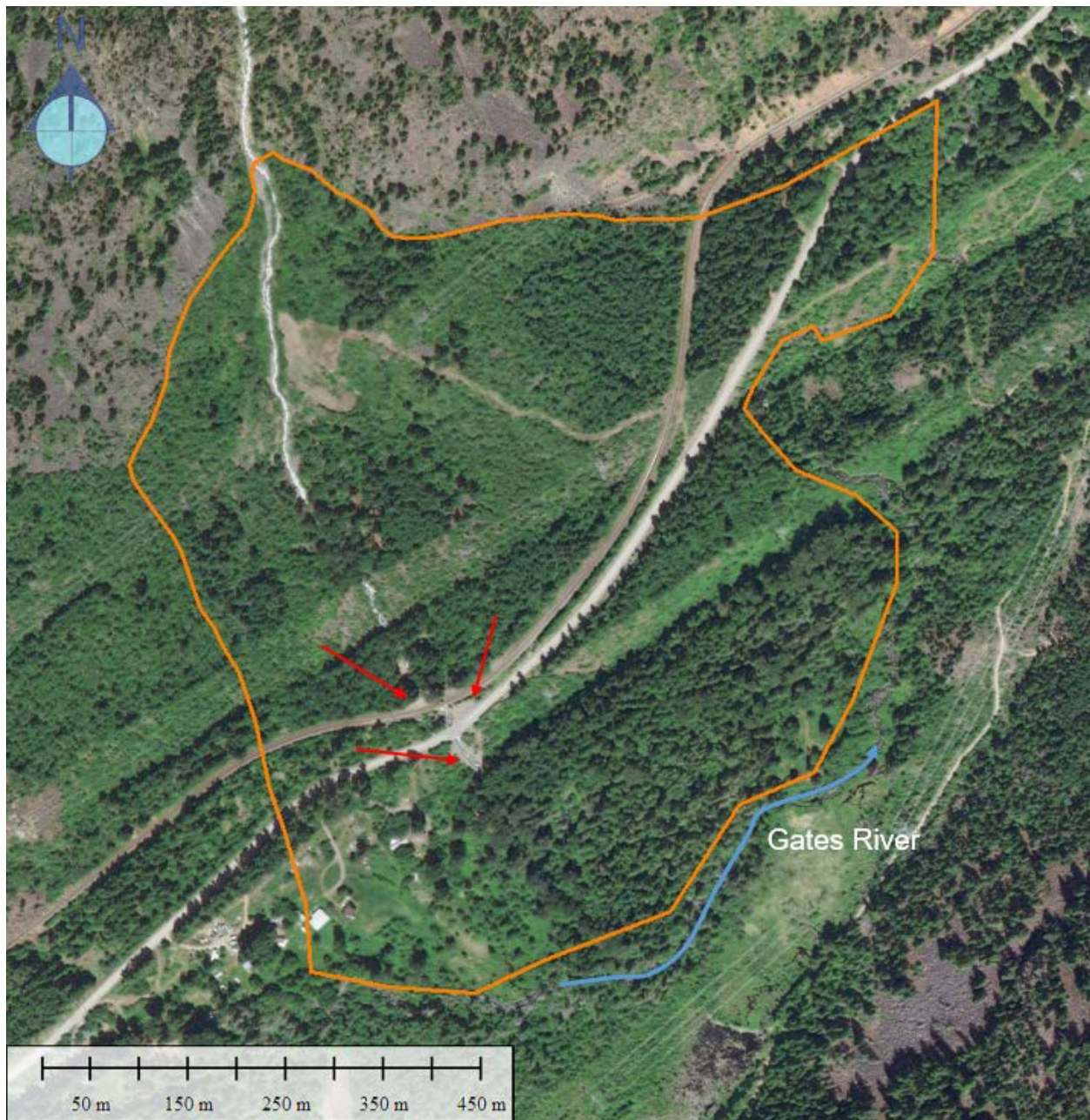
Figure E-12. Example of evidence (red arrows) for a recent (2015) debris-flow deposit on Neff Creek, located north of Pemberton. The approximate alluvial fan boundary is shown in orange (Imagery: DigitalGlobe, 2015).
