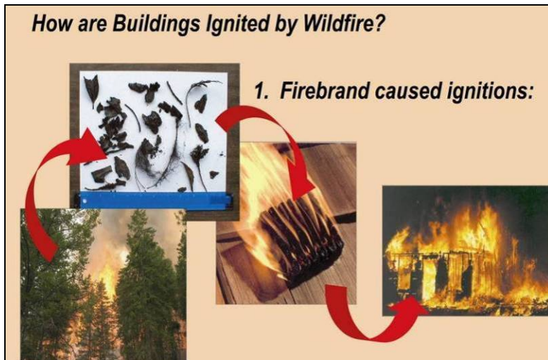
Figure 6. Firebrand caused ignitions: burning embers are carried ahead of the fire front and alight on vulnerable building surfaces or ignite surface fires which can threaten or destroy structures.
