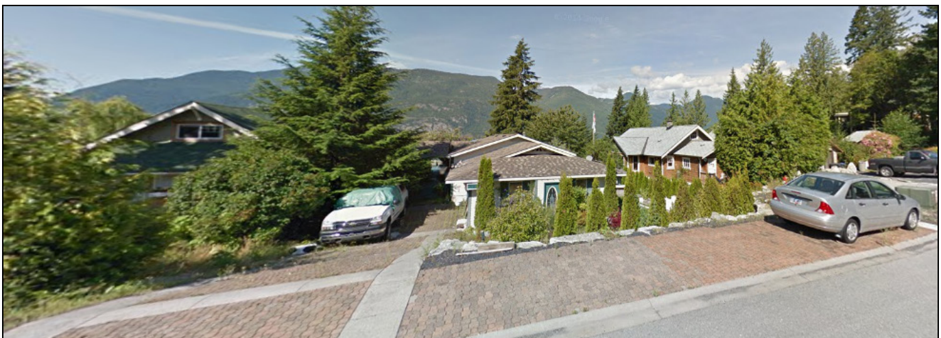
Figure 13. Britannia Beach: far left a home is obscured by both high and low-flammability vegetation in Priority Zone 1; middle a home with asphalt rated roofing, vinyl siding, and flammable hedging under the eaves; far right a home with rated roofing, cedar siding, and flammable hedging in front and side yards.
