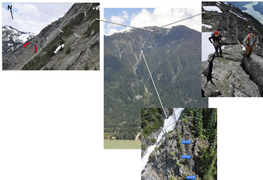
Photograph 20. Annotated photos showing potential landslide sources in upper basin area. White arrows show the location of the photos taken. Upper left: potential rock slide source on Lone Goat Peak. Upper right. Tension cracks on ridge crest. Lower center: toppling trees and tension cracks (arrowed) showing bedrock instability in the mid-basin area. Photograph taken by Matthias Jakob dated June 18, 2014
