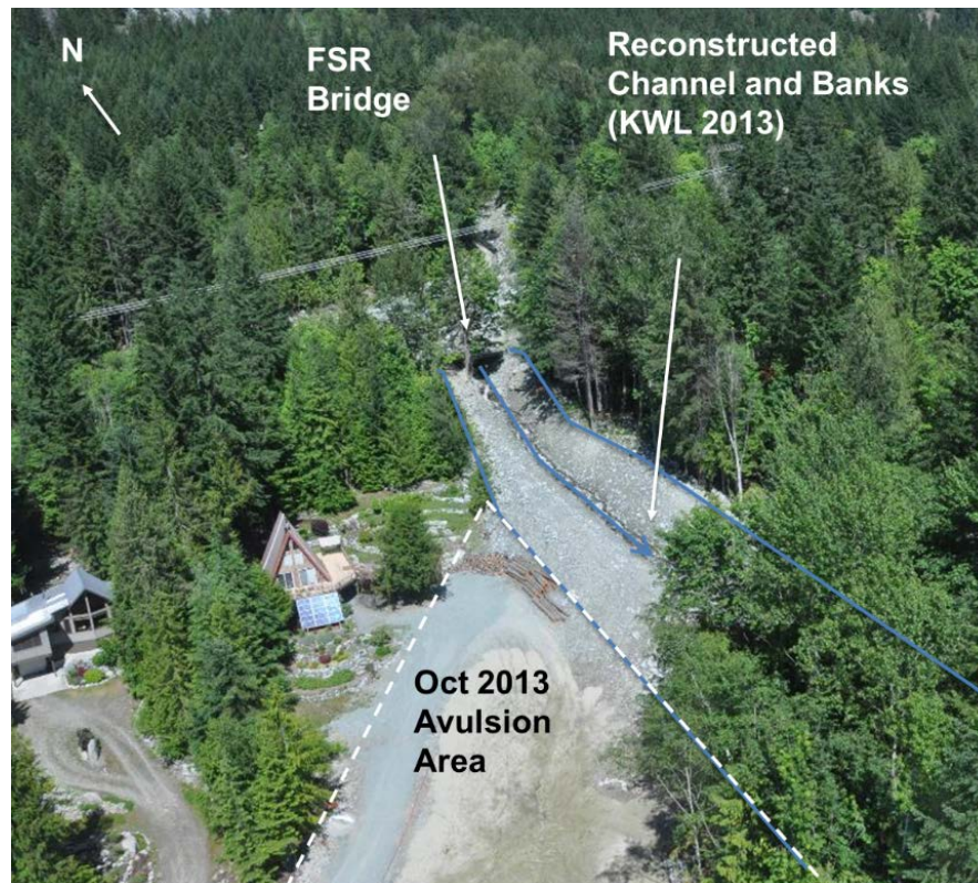
Photograph 15. Looking northeast at channel downstream of the FSR, showing the area of avulsion in October 2013. Photograph taken by Matthias Jakob dated June 17, 2014.
