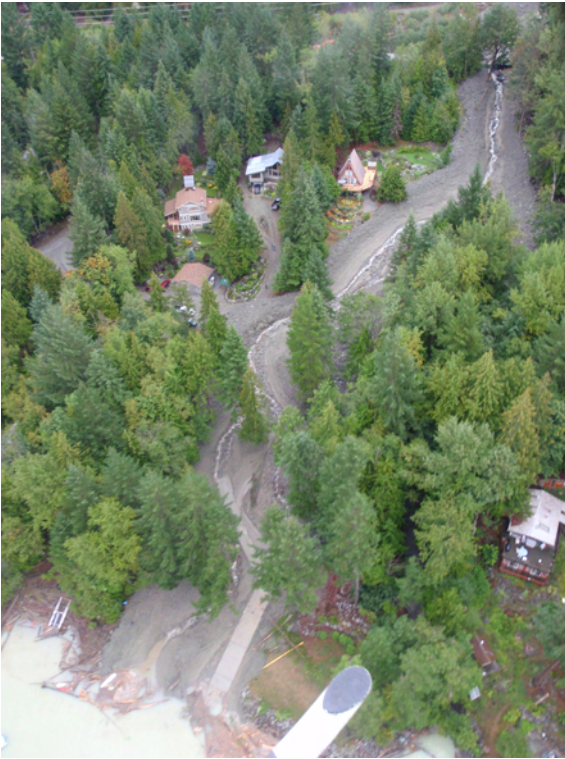
Photos 1 & 2. Aerial oblique NE views of the deposition zone below Lillooet Lake FSR. Note the southern lobe that triggered the northerly avulsion. The avulsing lobe missed the A-frame house by only a few metres. A pickup truck in the driveway was destroyed by the event and is likely in Lillooet Lake.
