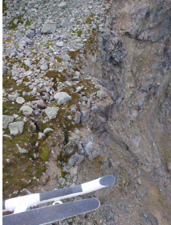
Photo 9. WP678. Area of tension cracking in bedrock. This site identified in 2010 represents a potential rockfall source area. Rockfall onto the debris blanket downslope could entrain significant volumes of additional debris.
