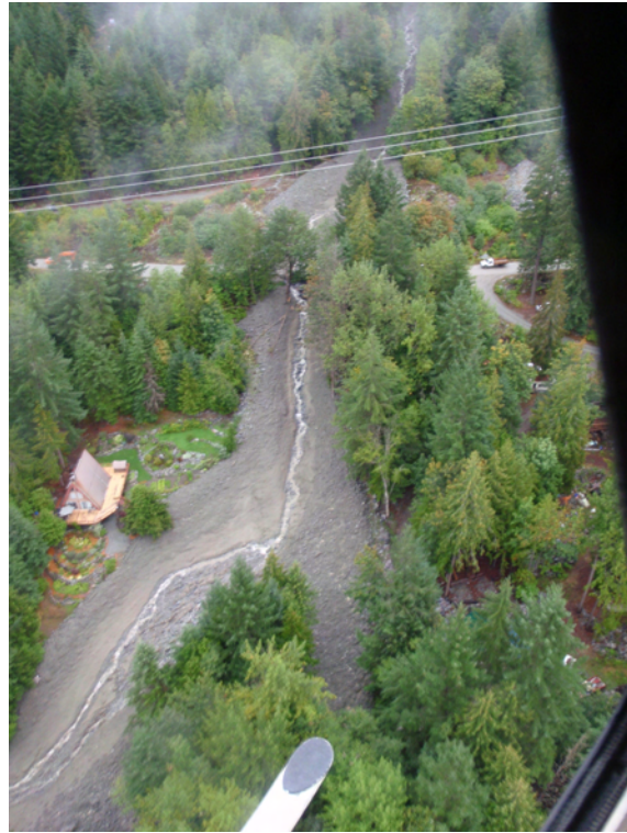
Photos 1 & 2. Aerial oblique NE views of the deposition zone below Lillooet Lake FSR. Note the southern lobe that triggered the northerly avulsion. The avulsing lobe missed the A-frame house by only a few metres. A pickup truck in the driveway was destroyed by the event and is likely in Lillooet Lake.
