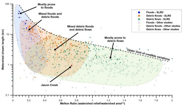
Figure 3-1. Steep creek process characterization based on watershed length and Melton Ratio. Note that this representation is simplistic because it does not include the dimension of return period. Some creeks are subject to different processes at different return periods.
