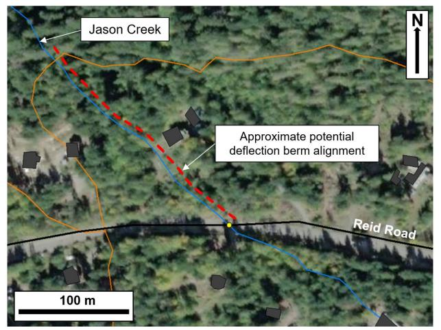
Figure 4-1. Approximate alignment of potential flow deflection berm (red). Jason Creek (blue line), fan boundary (orange line), building footprints (grey polygons), and Reid Road (black line) also shown. Base map is WorldImagery from Global Mapper.
