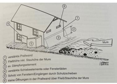
Figure 4-4. Example schematic of building-level risk control options. Annotations are in German and read 1) reinforced baffle, 2) flow height including the accumulation height of the mudflow, 3) buffer element, 4) reinforced sliding elements or shutters, 5) protection of windows/entrances with protective panes, 6) small openings in the impact wall above the flow/level of the debris flow. (Suda & Rudolf-Miklau, 2012). Other configurations are certainly possible.
